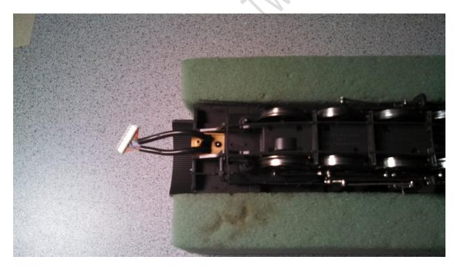
Re-attach the tender by reversing the disassembly steps.
