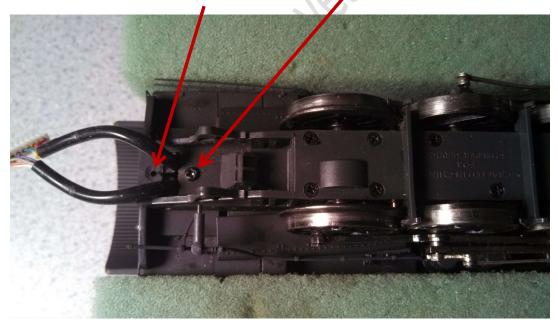
Next thread the plug and wires through the replacement brass bolster.
