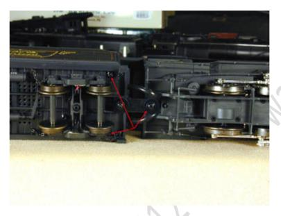
Turn the loco/tender upright on the table. The tender shell lifts straight off. Unplug the long connector with wires leading to the loco.
