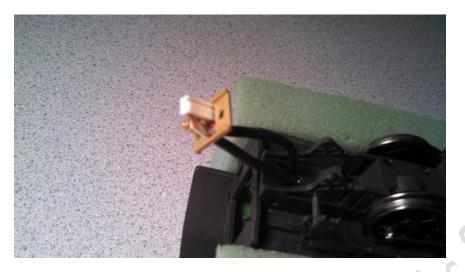
Slide the brass part down the wires and position on top of the plastic undercarriage. Re-install the screw removed in the previous step.
